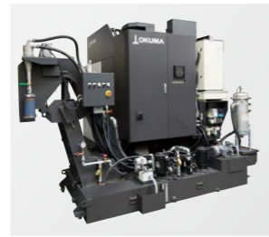
Sludgeless Tank (option)
