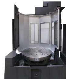
APC setup station
