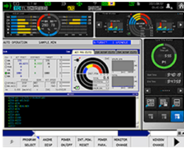
Figure 3: The ECO Power Monitor's operation screen, shown here on a 19-inch display.
